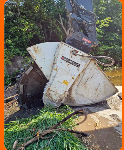
Close-up view of the KEMROC cutter wheel. It is designed to remove as much material from the concrete structure as is necessary for a clean cut.
